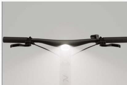
One-piece carbon handlebar intergrated with OLED display and LED Front 40LUX Light
