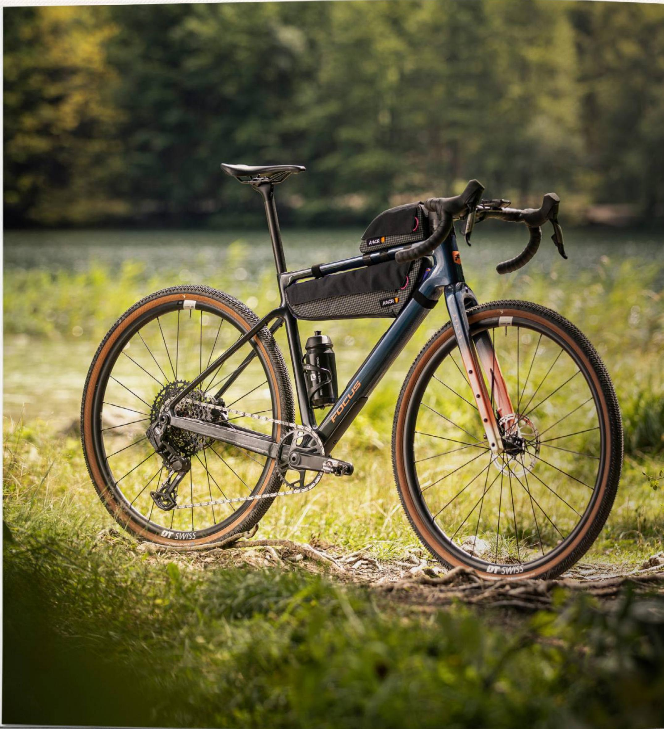
A Focus Atlas 8.8 gravel bike is shown from a three-quarter front angle, leaning slightly to the left. The bike has a dark frame with orange accents, a carbon fork, and DT Swiss wheels. It is equipped with a flat-mount disc brake system and a SRAM Eagle drivetrain. A black ACR bag is mounted on the seat stay. The background is a blurred green forest.
