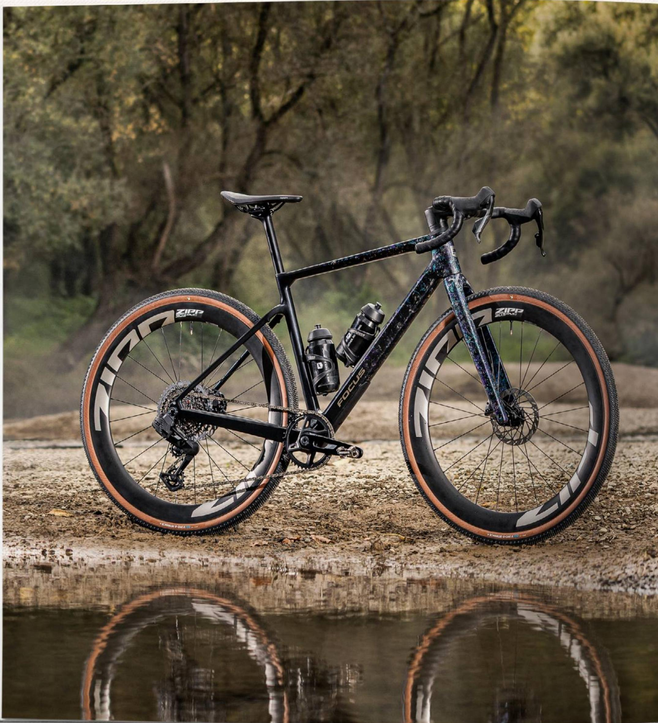
A black Focus Atlas 8.9 gravel bike is shown from a three-quarter front angle, leaning slightly against a tree trunk. The bike features a dark frame with orange highlights, Zipp Service Course SL 70 XPLR wheels, and Schwalbe G-One R Pro tires. It is equipped with SRAM Rival E1 AXS drivetrain and disc brakes. Two water bottles are mounted on the frame. The background is a blurred autumn forest.
